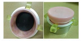
Put 500 grams of weight into the empty solder paste cups, easy to remove, in order to better protect the aluminum mixing cup is not damaged
